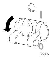
2. Check to be sure the power switch is in the off position (down).
